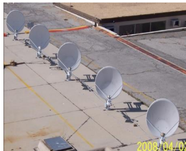
Fig. 10 2009 NASA JPL array study, 5 1.2m offset paraboloid antennas “Calibration Tower Method”
