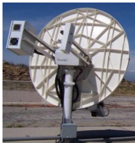
Fig. 9 2009 NASA JPL array study Left side counterweight carries DC power supplies for the electronics
